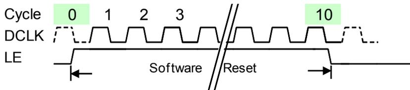
“Software reset” command makes MBI5155 go back to the initial state except configuration register value. After this command is received, the output channels will be turned off and will display again with last gray-scale value after new “Vsync” command is received.
