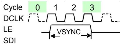
“VSYNC” command is used to update frame data on output channels ( $\overline{OUT0}$ ~ $\overline{OUT15}$ ). There are some timing limitations between signal “LE” and “GCLK”; and please refer to the section of “Vsync Command Operation” for details.
