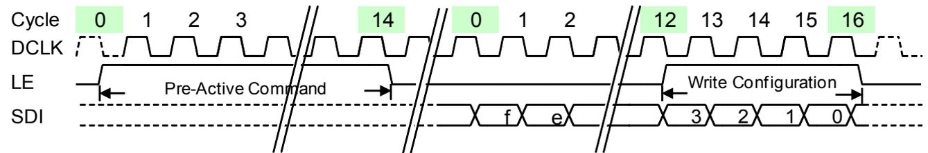
“Write configuration” command is used to program the configuration register of MBI5155. The “Pre-Active” command must be sent in advance. When this command is received, the last 16 bits data before the falling edge of LE will be latched into configuration register, as shown in the above waveform, and MSB bit needs to be sent first.
