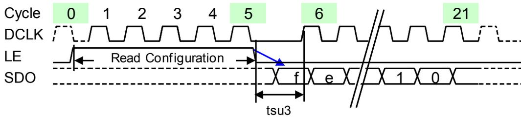
“Read configuration” command is used to read the configuration register of MBI5155. When this command is received, the 16-bit data of configuration register will be shifted out from SDO pin, as shown in the above waveform, and MSB bit will be shifted out first.
