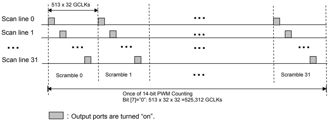
GCLK multiplier enabled (configuration register1 bit [6] = 1)
