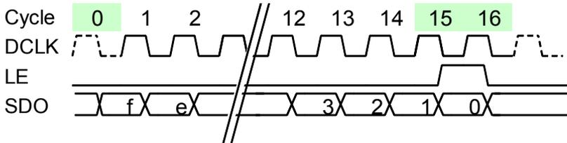
Data Latch command is used to latch the 16-bit shift register from SDI to internal SRAM buffer. When this command is received, the last 16 bits data before the falling edge of LE will be latched into SRAM, as shown in the above waveform, and MSB bit needs to be sent first.
