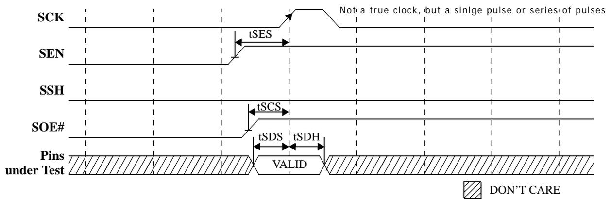
**Figure C-3: Scan Shift Timing**
