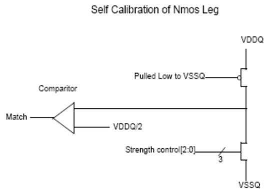
When Match Nmos leg is calibrated to 240 ohms
