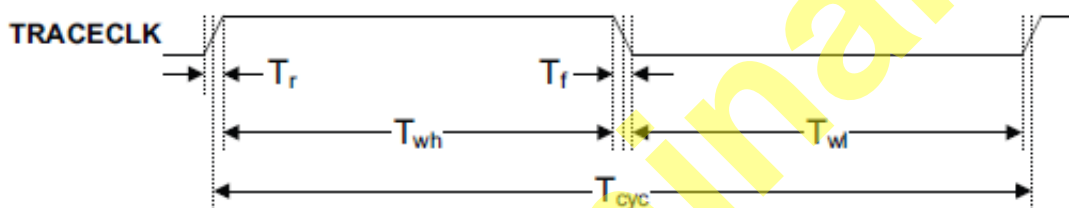
Figure 3. TRACE_CLKOUT specifications
