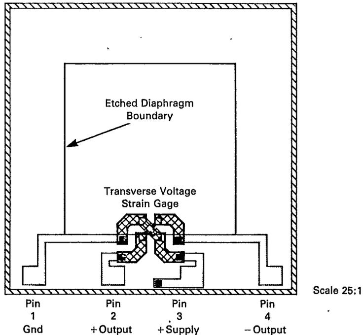
**FIGURE 3 — MPX PRESSURE SENSOR ELEMENT CROSS SECTION (DIFFERENTIAL)**
