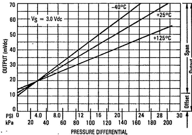
OPERATING CHARACTERISTICS ( $V_S = 3.0 \text{ Vdc}$ ,  $T_A = 25^\circ\text{C}$  unless otherwise noted.)
