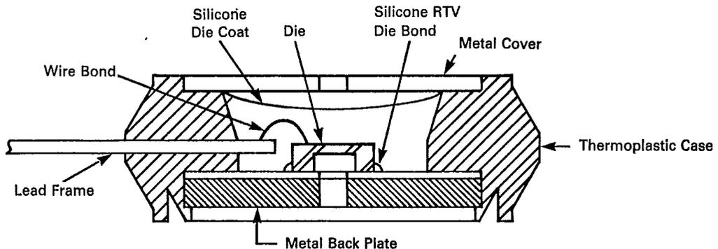
Figure 3 shows the cross section of the Motorola MPX pressure sensor die in the chip carrier package. A silicone gel isolates the die surface and wire bonds from
