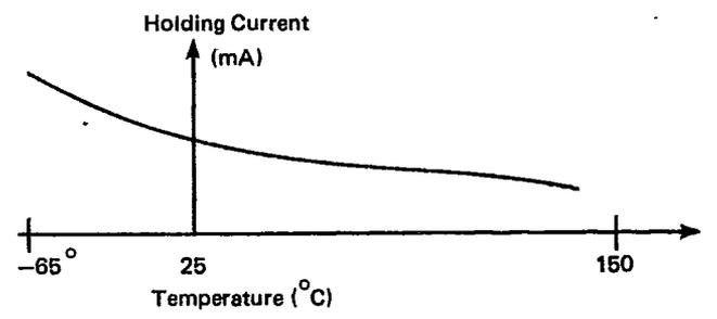
The change in Ih with temperature can be reduced but other parameters e.g. T on are increased.
