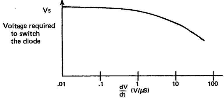
The shape of the above can be controlled and the diode can be designed with no change up to 10 V/us.
