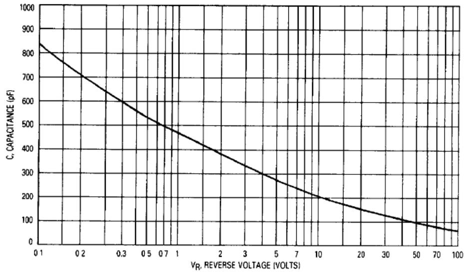
**Figure 7. Typical Capacitance (Per Leg)**
