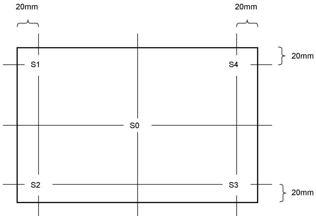
$$\text{Standard Value of Brightness Uniformity} = \frac{\text{Minimum Value of S1-S4}}{S0}$$
