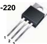
1.Gate 2. Drain 3. Source
